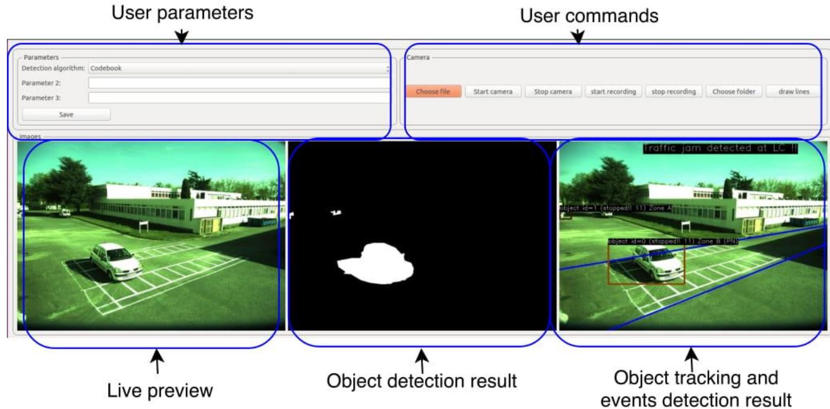
A fully smart detection system based on video sensing and image processing
