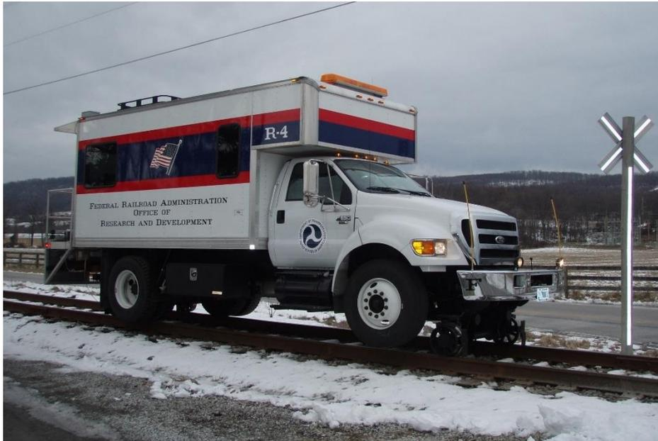
LiDAR Surveying System to be installed on the Hi-Rail "R4" research vehicle.
