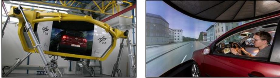
**Figure 4:** DynSim (Dynamic Driving Simulator)
