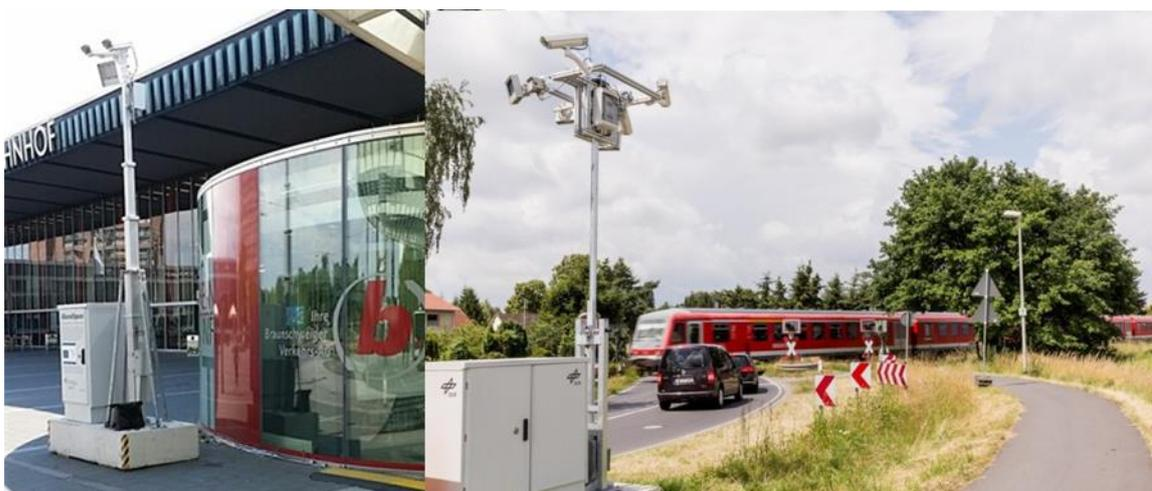
**Figure 26:** Mobile sensor poles at railway station and level crossing
