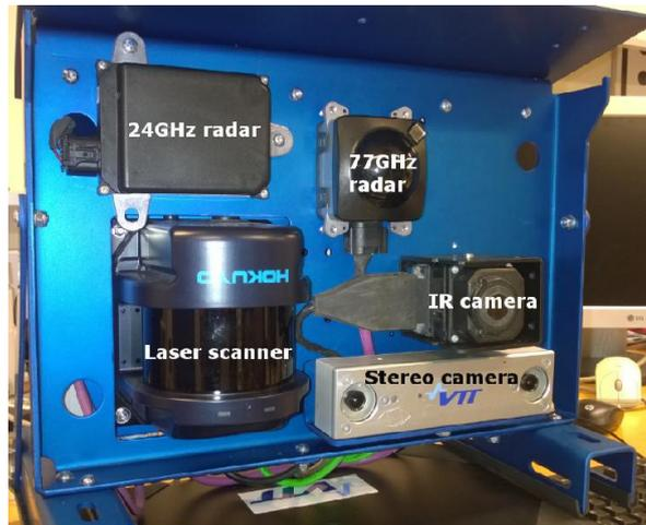
**Figure 21:** Portable sensor rack for rapid prototyping and feasibility tests. © VTT
