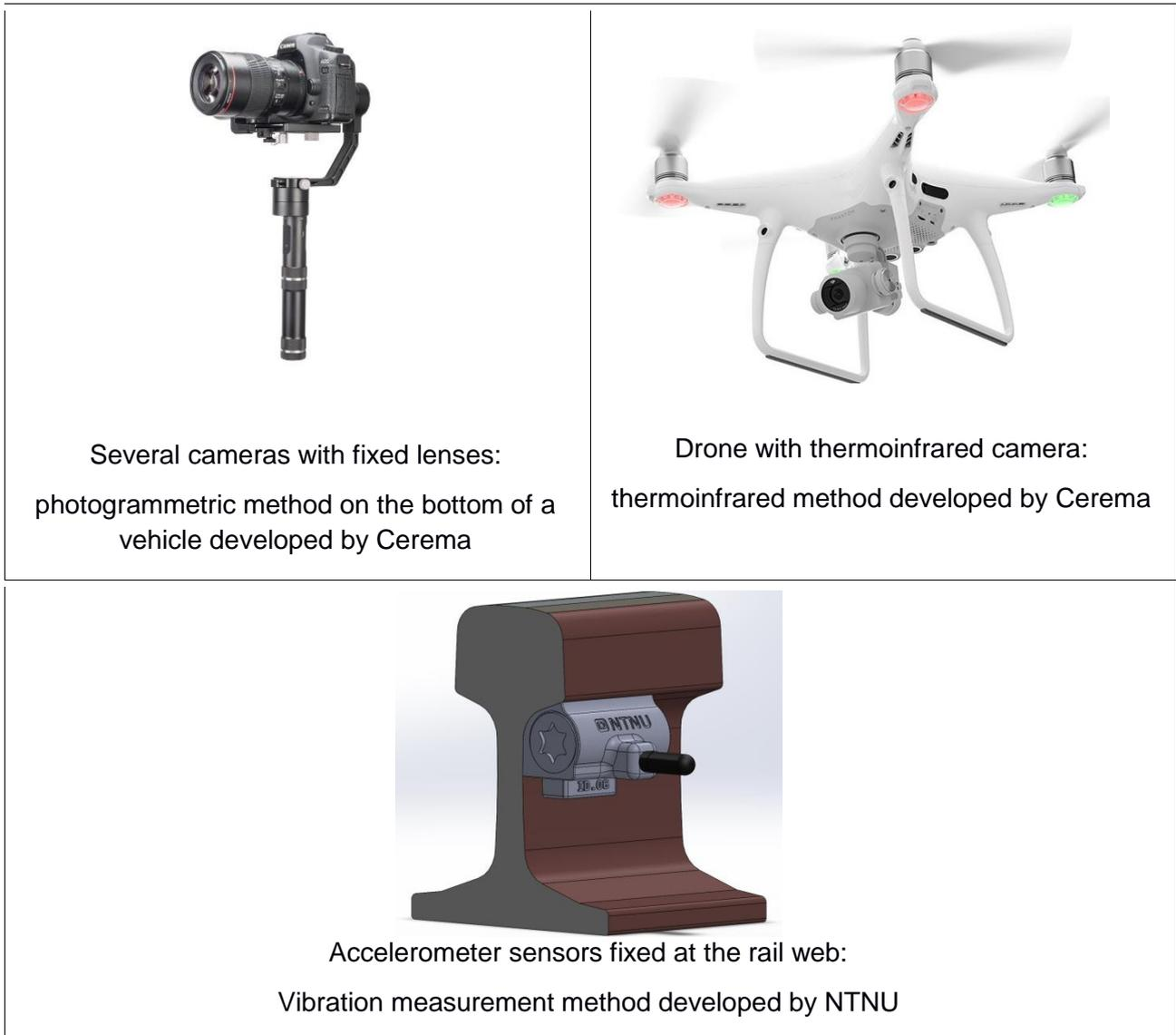
**Figure 14:** Measurement tools to be used in the Cerema test site
